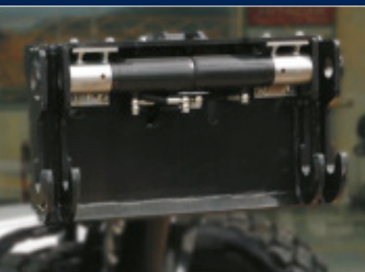
Quick coupling flange with hydraulic locking pins
