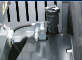
Auxiliary hydraulic socket with quick coupling
