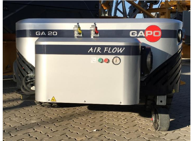
AIRFLOW (compressor for semi-trailers braking system)
