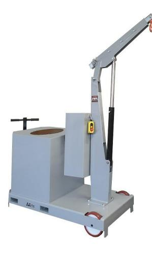
GZ1000BP is equipped with a pendant lever for lifting a load at a single speed and operating a progressive descent . This requirement is indispensable when millimeter accuracy is required during the positioning of the load.
